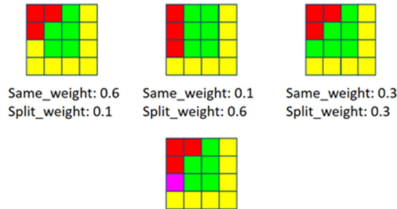
Fig.5.The voting algorithm (top: an over-segmenting algorithm, an under-segmenting algorithm, and a balanced algorithm; bottom: the voting result).
